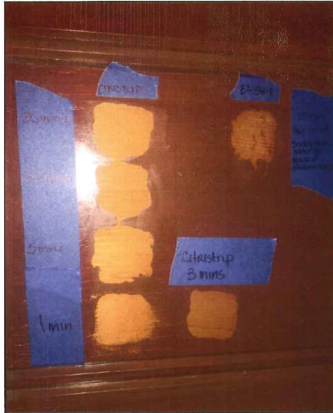
Image 28: Test samples of coating removal treatments showing exposed sugar pine wood cladding following removal of existing discolored clear coatings (Biddle, 2016)
